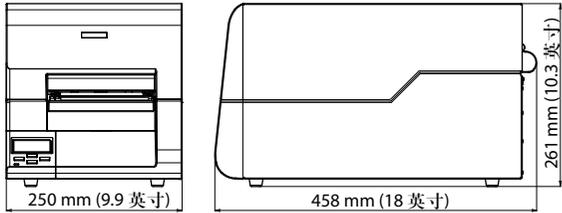
The image contains two technical drawings of the printer. The left drawing is a front view showing the printer's internal components like the paper tray and print head. Below it, a dimension line indicates a width of 250 mm (9.9 inches). The right drawing is a side profile view of the printer, showing its depth and height. Below it, a dimension line indicates a depth of 458 mm (18 inches), and on the right side, a vertical dimension line indicates a height of 261 mm (10.3 inches). |
